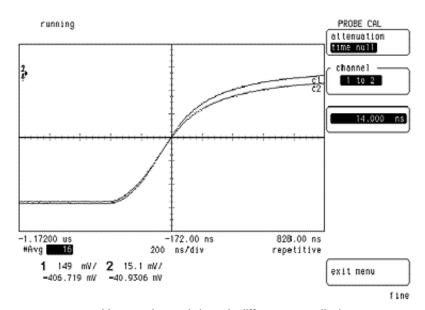
Note probe path length differences nulled out.
