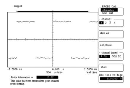
Note the Probe Attenuation factor shown on screen.
